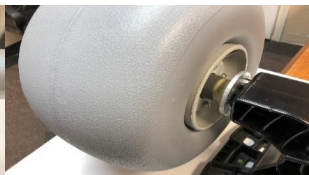
8. Install WheelEEZ® Balloon Wheel over Axle Extender.
