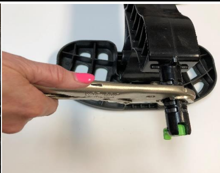
2. Use vise grip pliers to twist and pull off plastic portion of axle.
