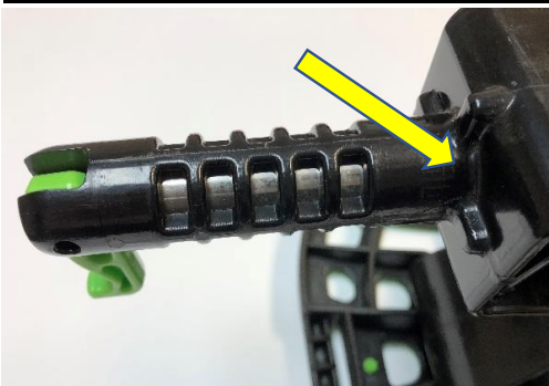
1. Use hacksaw, carefully cut around entire plastic axle portion only.
